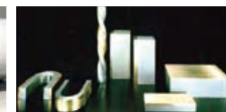
Clad steel plates
